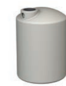
BT900 900L/200gal Height 1,450mm Diameter 1,000mm Outlet 25mm Overflow 50mm
