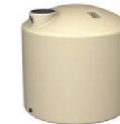
BT5000-S 5,000L/1,100gal (Squat) Height 1,900mm Diameter 2,000mm Outlet 25mm Overflow 90mm Inlet 1,850mm
